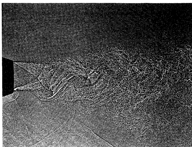
Fig. 2 Supersonic jet shadowgraphs of sound incidences on jet boundary: a) head on, \alpha = 30 deg and b) oblique, \alpha = 160 deg; n = 0.8 .
